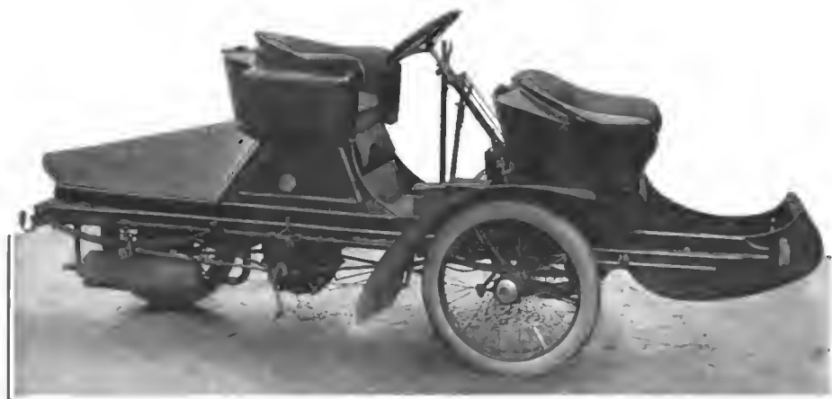
ENGLISH TRI-CAR WITH 8-HORSEPOWER, TWO-CYLINDER ENGINE AND AUTOMOBILE SPRINGS.
